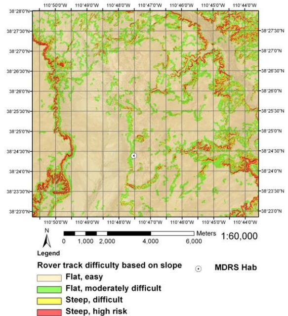
**Figure 4:** Early results illustrate rover track difficulty based on slope.
