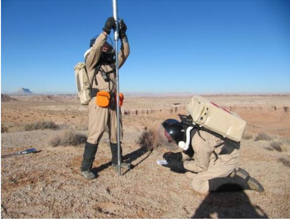
**Figure 2:** Crew conducts blowcount test with the cone penetrometer
