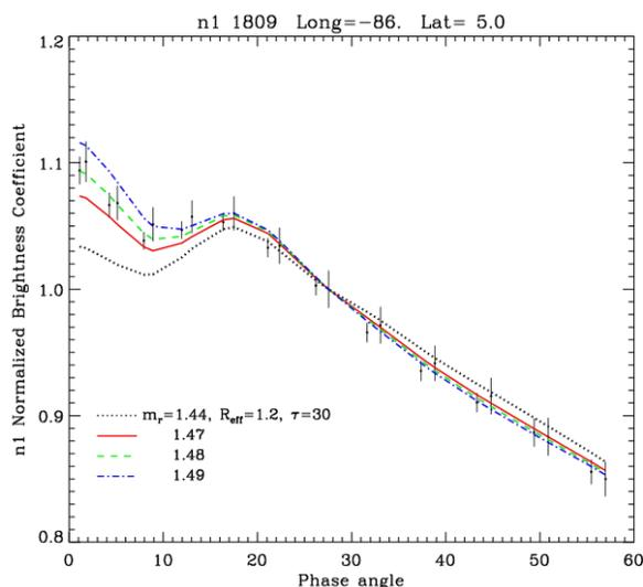
Figure 3. Measured NIR brightness compared with the model of cloud layer composed of mode-2 particles with various values of the refractive index.
