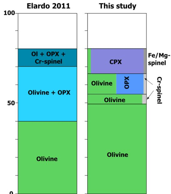
**Figure 2** Block diagram showing the experimentally determined cumulate pile under equilibrium (left hand side – [6]) and fractional (right hand side – this study) conditions. The equilibrium assemblages are estimated based on the dominant assemblage crystallizing at each depth in the experimental study. The two scenarios show a marked difference in pyroxene abundance and composition, with the fractional case producing aluminous spinel and calcic pyroxene much earlier in the sequence.
