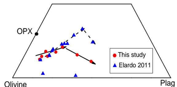
**Figure 3** Liquid line of descent in the equilibrium and fractional case. Silica is at the apex of the ternary. The equilibrium experiments [6] (blue triangles, dashed line) produce a melt less enriched in the plagioclase component and more enriched in silica than the fractional experiments (red circles, solid line).
