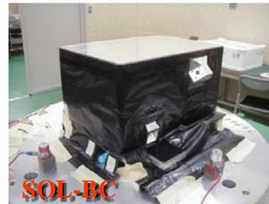
**Figure 2.** Kaguya SOL-BC on the mechanical test. SOL-C is part of this component with a standard sample.
