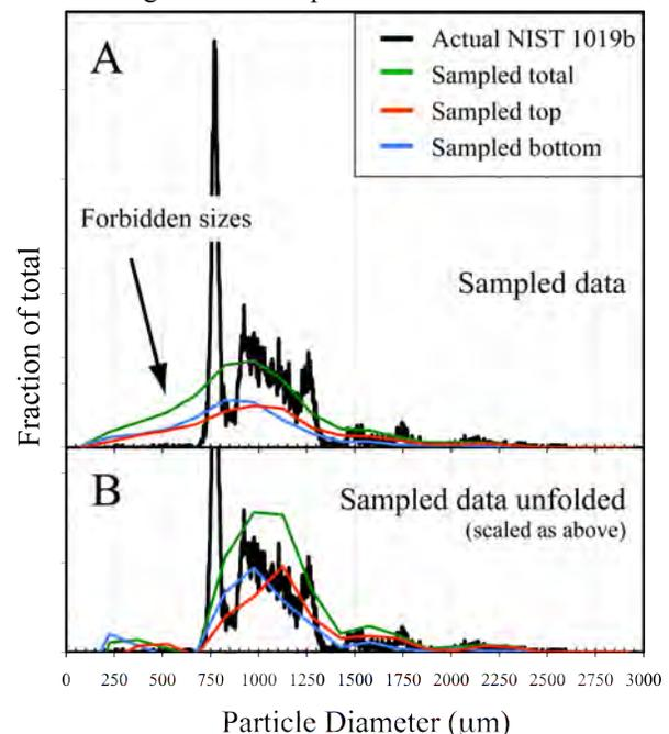
**Figure 4.** Top panel shows the line histogram data generated from measurements of NIST 1019b. Bottom slice data is in blue, top slice data is in red, total slice data is in green, and the accepted values are in black. Bottom panel shows data after unfolding. Note that the settling shows up clearly as does the modes of the larger particles.
