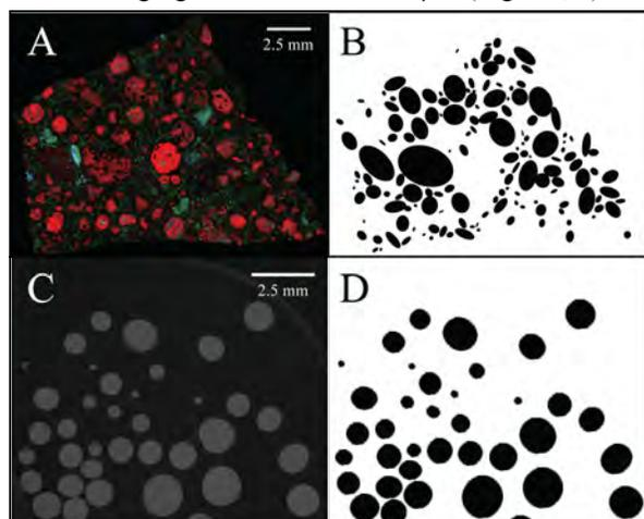
**Figure 1.** A) X-ray chemical map of Allende, with Mg, Ca, and Al as red, green, and blue. B) Best fit ellipses defined by ImageJ for just porphyritic chondrules from A. C) An example radial section of the NIST 1019b particle size standard imaged by x-ray tomography [10]. D) Best fit ellipses defined by ImageJ of glass beads from C.
