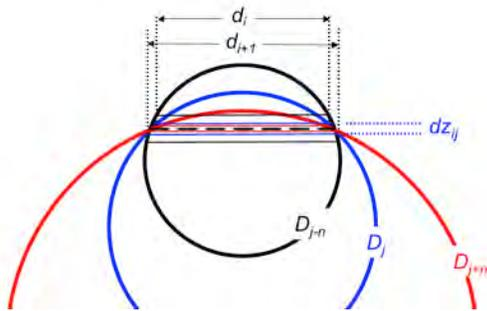
**Figure 3.** Graphical representation of the unfolding problem. The size distribution  $N_A(d)$  and  $N_V(D)$  are binned the same way, into a set of diameter bins with lower and upper boundaries at  $(d_{i-1}, d_i)$ , with  $i = 1$  representing the top end of the smallest particle size bin. For simplicity, we assume the spacing is regular, so  $d_i = d_{i-1} + \Delta$ , with  $\Delta = D_{\max}/N$ .
