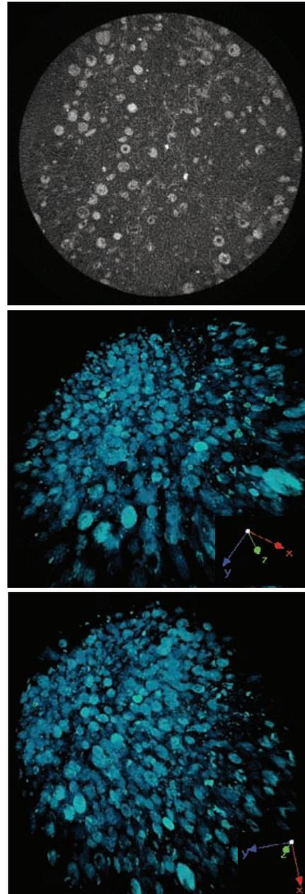
**Figure 3:** MicroCT images of spherules from a core of the S3 bed. Image to the upper left shows a single raw image of the core. Diameter of the circle is 1 inch. The two other images show the thresholded and processed data rotated to three orientations (x, y, and z axis shown in lower right for each image).
