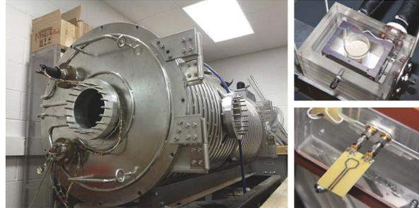
**Fig 4.** (Left) The MMEC Vacuum Chamber. (Right, top) A small sample chamber with 250 mL soil sample. (Right, bottom) The microwave soil moisture sensor.
