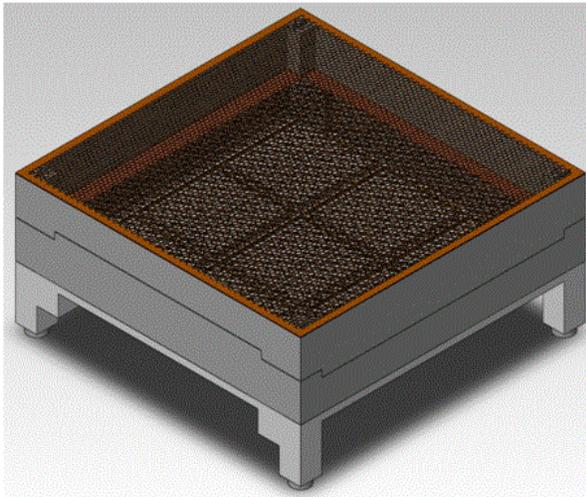
*Fig.2 Piezo Dust Detector: Main detector unit with 9 piezo sensor elements and 2 grids.*
