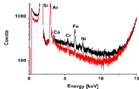
Figure 4: Spectra of a 1kV (black) and 2 kV (red) Mg Ca Cr implants in silicone after CO<sub>2</sub> snow cleaning.
