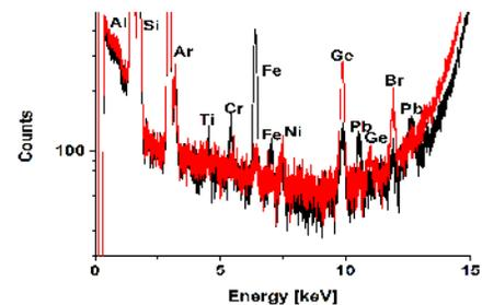
Figure 1: TXRF spectra of Genesis sample 60966 (silicon on sapphire) before CO<sub>2</sub> snow cleaning (black) and after CO<sub>2</sub> snow cleaning (red).
