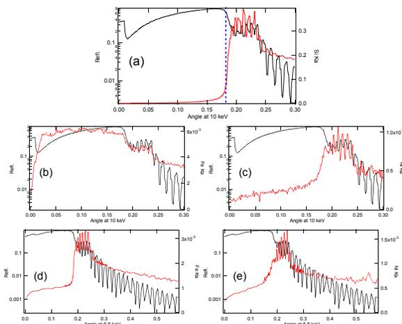
Figure 3: Total reflectivity of X-ray beam (black) and fluorescence yield (red) as a function of incident X-ray angle in degrees. Si
