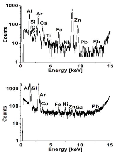
Figure 2: TXRF spectra of sample 60326 before cleaning with concentrated HCl (left) and after (right).
