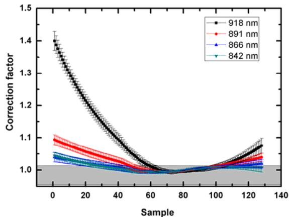
Fig. 3. The empirical correction factors derived for four IIM bands by using 15 standard lines
