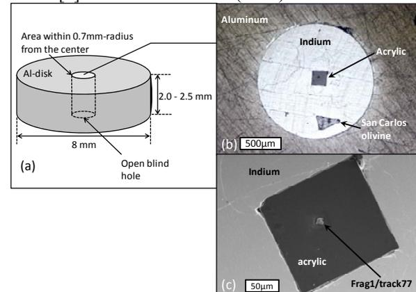
**Fig. 1:** A schematic drawing of an Al-disk (a), an optical microscope image of a Wild 2 particle (fragment 1 from track 77; [4]) (b), and a secondary electron (SE) image of the fragment 1 from track 77 (c).
