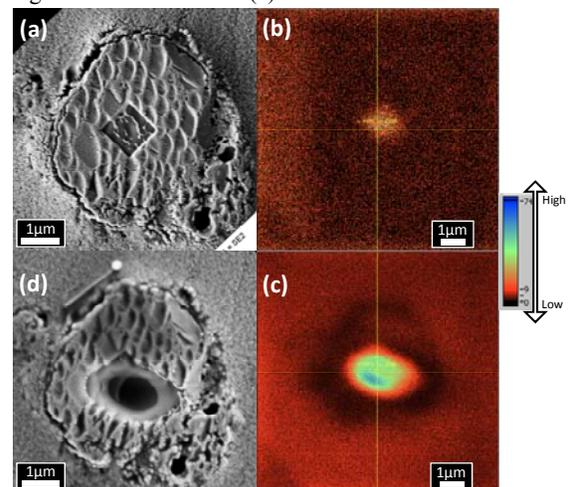
**Fig. 2:** SE image of a Wild 2 particle (fragment 4 from track 77; [4]) before the oxygen isotope analysis (a),  $^{16}\text{O}^-$  ion image before the oxygen isotope analysis (b),  $^{16}\text{O}^-$  ion image after the oxygen isotope analysis (c), and SE image of fragment 4 from track 77 after the oxygen isotope analysis (d).
