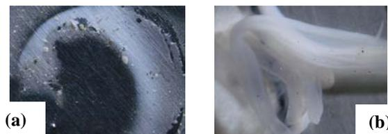
**Figure 1.** Microscopic image of  $\text{SiO}_x$  formed in the laser plume in gas phase: (a) the white  $\text{SiO}_x$  formed on the bottom plate of the reaction chamber; (b)  $\text{SiO}_x$  formed underneath the  $\text{MgF}_2$  window of the reaction chamber.
