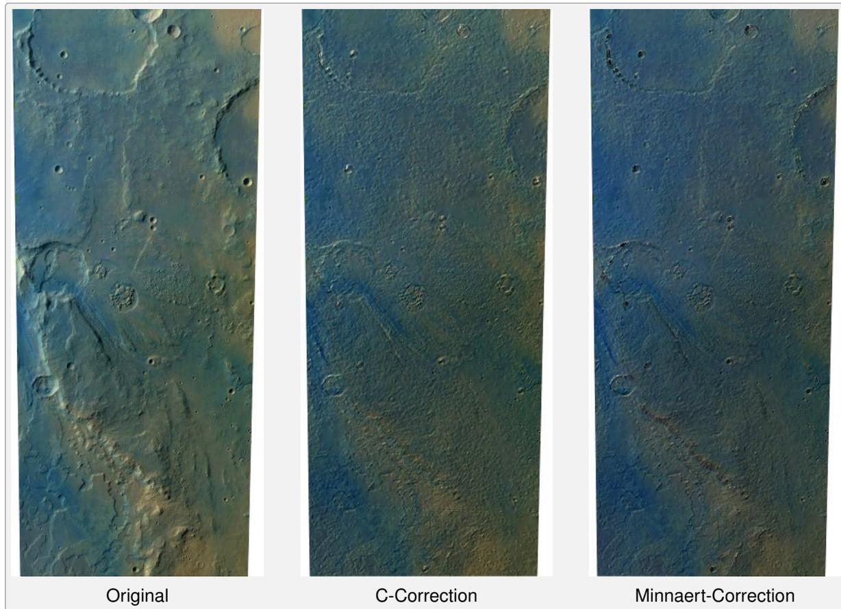
Figure 2: comparison of the original HRSC sequence of orbit 901 (left) and the topographically corrected images (middle and right). A contrast-stretched false color representation of the HRSC scene has been chosen.
