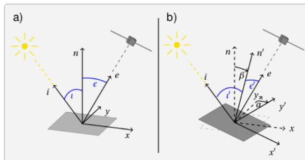
Figure 1: horizontal surface element illuminated by angle  $i$  and observed by angle  $e$  (a). The inclined surface element has the effective angles  $i'$  and  $e'$  (b).
