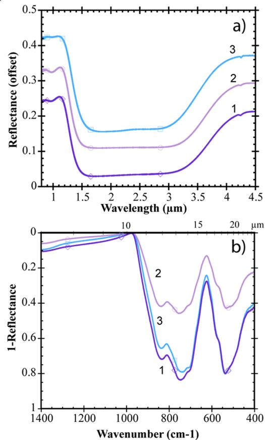
**Figure 3:** Reflectance spectra of Spinel 1, 2, and 3 in a) NIR and b) MIR wavelengths. A prominent 2-3  $\mu\text{m}$  absorption is present in all run products, but the 1  $\mu\text{m}$  band is only present in the spinels with FeO  $\geq 5\%$ .
