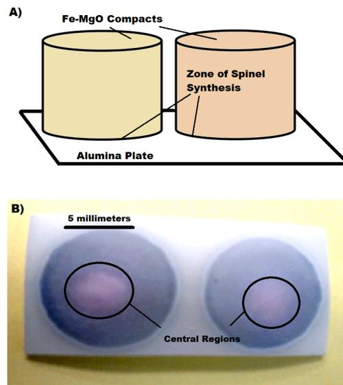
**Figure 1:** A) Diagram of experimental setup and B) picture of representative run products. Compacts with different Fe/Mg (represented by different color in 1a) were placed on alumina plates. The central regions are the areas where the compacts remained in direct contact with the plate for the duration of the experiment. These are the regions where the reported spinel spectra were taken.
