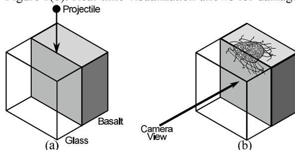
**Figure 1. Schematics of: (a) bonded basalt/glass specimen, (b) bonded basalt/glass specimen showing camera location to view damage through glass.**
