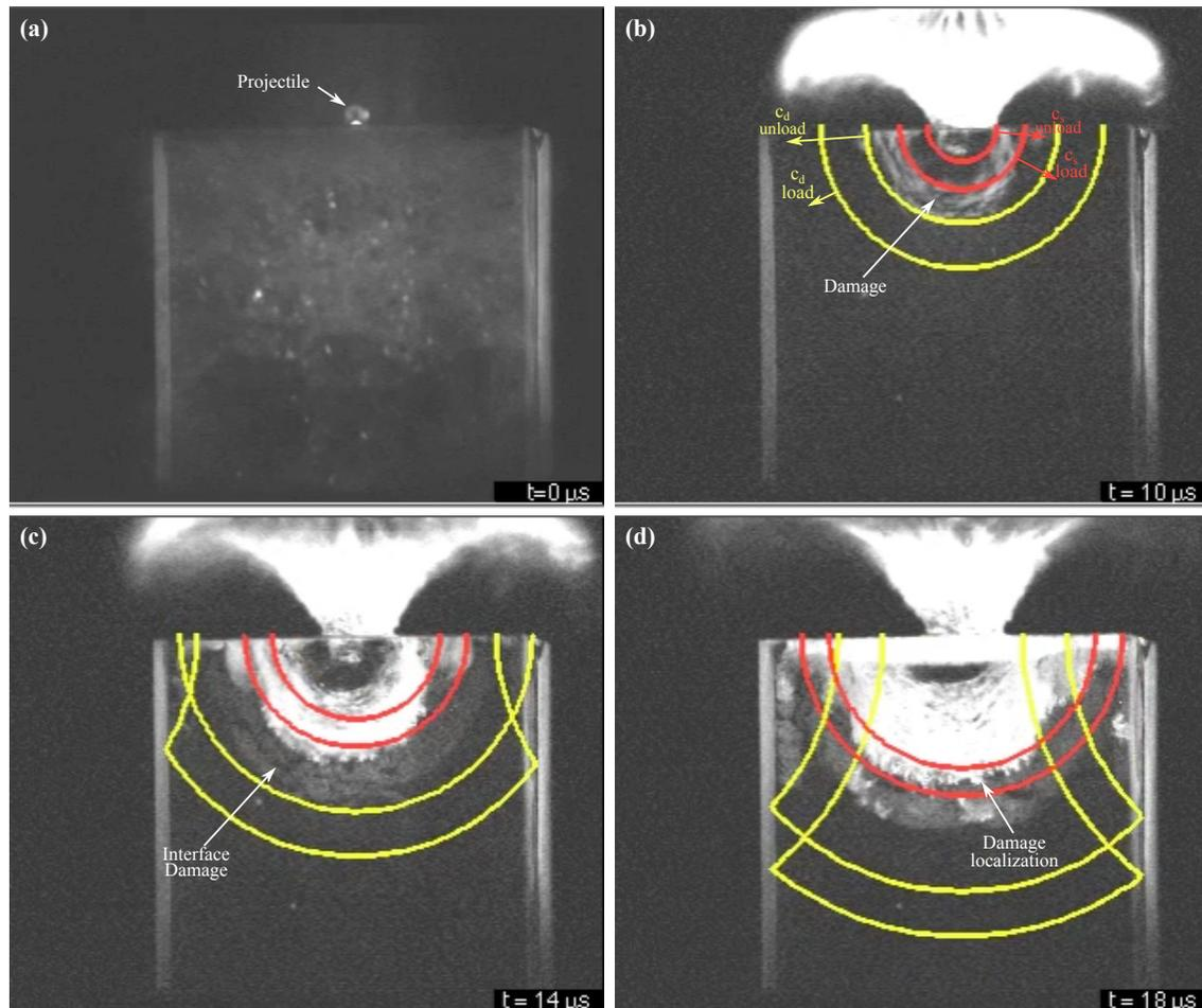
**Figure 2. High-speed images captured during a 3 km/s impact on a basalt/glass target. Camera is aligned so that view is through the glass focusing on the interface between the two materials.**
