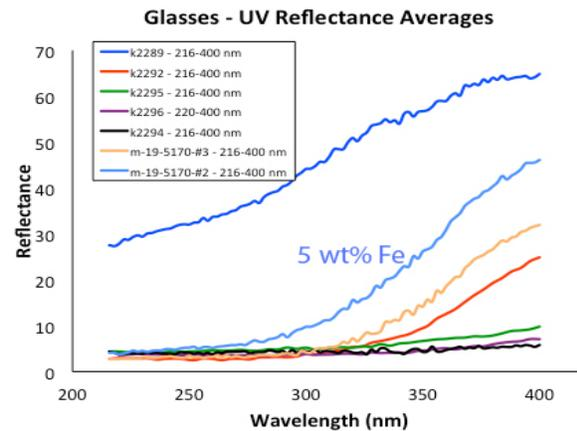
Fig. 5. Laboratory spectra of glass samples [12], from iron-free (dark blue) to 22 wt% Fe (purple and black). The UV-VIS slope of low-iron glasses, similar to those for low-iron pyroxenes [10,11], are consistent with VIRS spectra. Higher iron contents have less steep UV absorptions and overall lower reflectance.
