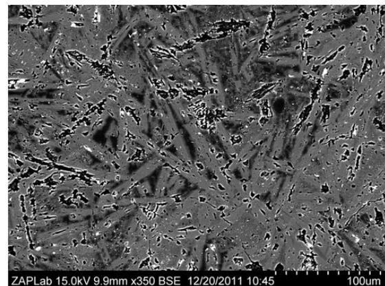
**Fig. 2.** BSE SEM image of the red impact melt rock showing the fine-grained groundmass comprised of K-feldspar laths (pale grey) and glassy mesostasis (dark grey).
