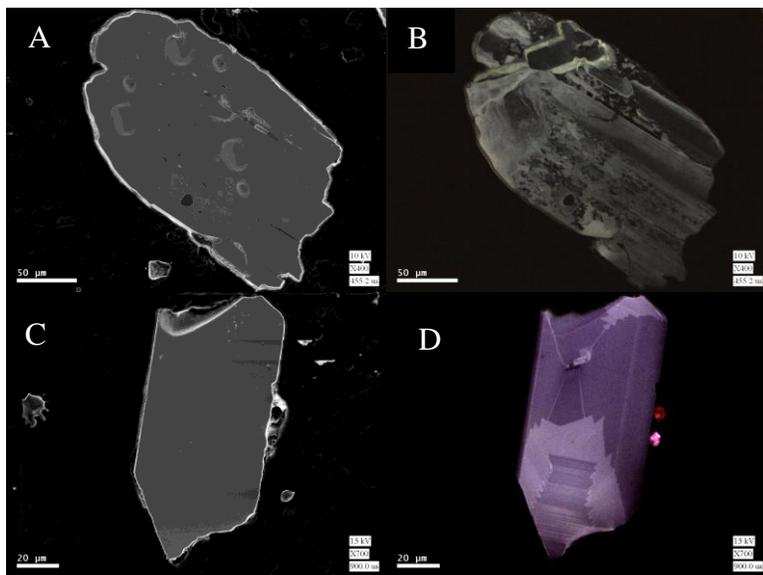
Figure 1: Sectioned, polished zircons from a gabbro-norite body near the center of the Vredefort dome showing the difference between shocked and unshocked grains. (A & B) SE and CL images of a grain that has been shown to have been shocked and recrystallized using CL and electron backscatter diffraction strain mapping [9]. (C & D) SE and CL images, respectively of an unshocked, igneous grain from the largest body of gabbro-norite with typical oscillatory planar growth banding and sector zoning.
