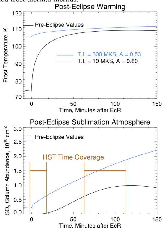
**Figure 2** Temperature, from a 1-D thermophysical model, and resulting equilibrium sublimation  $\text{SO}_2$  column density over the period of our observations, for two very different assumptions about the frost thermal inertia ( $T.I.$ ) and albedo ( $A$ ), chosen to give similar pre-eclipse temperatures. Column densities are calculated on the assumption of instantaneous vapor pressure equilibrium with surface temperature- dynamic processes may result in a slower response.
