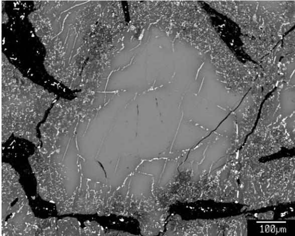
**Figure 4:** Backscattered electron (BSE) image of a reduced olivine grain found in our coarse grained ureilite sample. Core =  $Fa_{20}$  and rim =  $Fa_3$ . White blebs = Fe metal. Large black patches = a carbon phase. Smaller black regions = cracks and pits.
