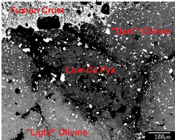
**Figure 5:** BSE image of various phases in our fine-grained ureilite sample. Low-Ca Pyx =  $En_{86}Fs_9Wo_5$ , "Dark" Olivine =  $Fa_{12}$ , and "Light" Olivine =  $Fa_{18}$ . White blebs are metal. Black patches are either a carbon phase or voids/pits/cracks. A patch of fusion crust is shown at the top left of the image.
