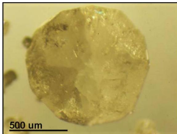
**Figure 1. Reflected light microscope image of synthetic whitlockite crystal grown as part of this study.**
