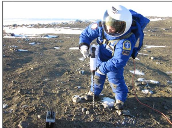
Figure 2: The NDX-1 was used to gather subsurface samples and radiation data on Marambio Island.
