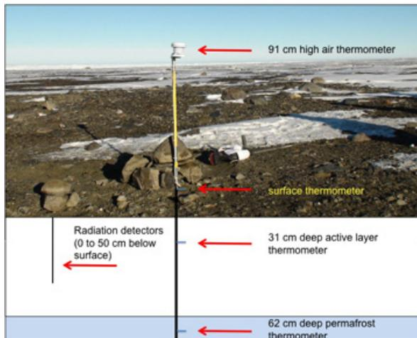
Figure 3: The Marambio surface and subsurface climate monitoring station is located on a rocky surface at 64°S 14.783', 56°W 39.131.
