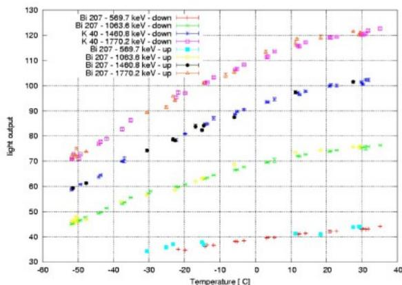
Fig. 3: The temperature dependence of the CsI scintillator can be accurately characterized. The different curves show the response of CsI to various lines of  $^{207}\text{Bi}$  and  $^{40}\text{K}$ .
