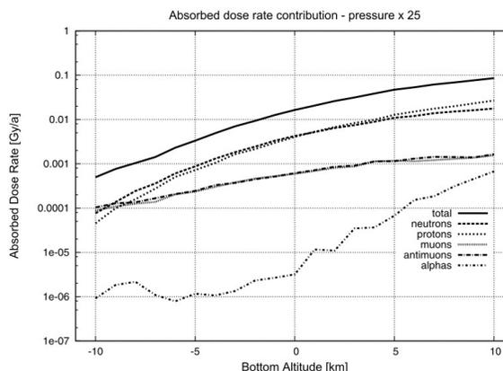
Fig. 5: Altitude dependence of the various particle species contributing to the dose rate at the Martian surface for an atmospheric pressure 25 times today's. From [2].
