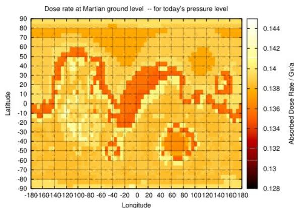
Fig. 4: Absorbed dose rates on the Martian surface for present-day conditions. These were different and higher in the past when Mars had a thicker atmosphere. From [2].
