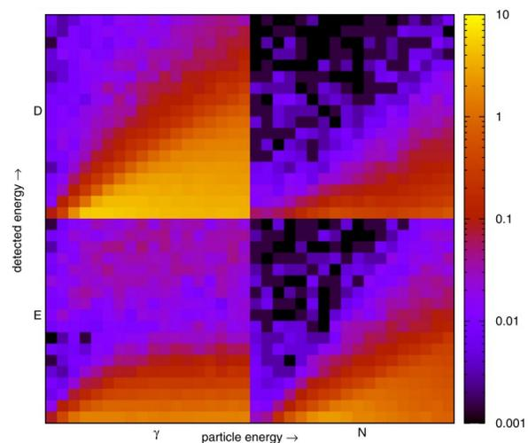
Fig 2: RAD geometric factor for neutrons (right) and gammas (left) in CsI (top) and BC432m (bottom). From [1].
