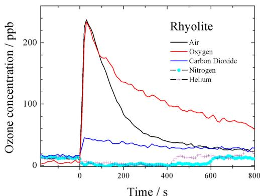
phere was pumped into the ozone detector through particle filter. Initially, the ozone signal increases due
