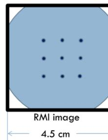
**Figure 2** Schematic geometry for a Recon Grid analysis with nine points 1 cm (5 mrad) apart at 2 m range. Spacing to as little as 400  $\mu$ m between points is possible. Pre- and post-LIBS RMI images are co-registered with the central analysis point.
