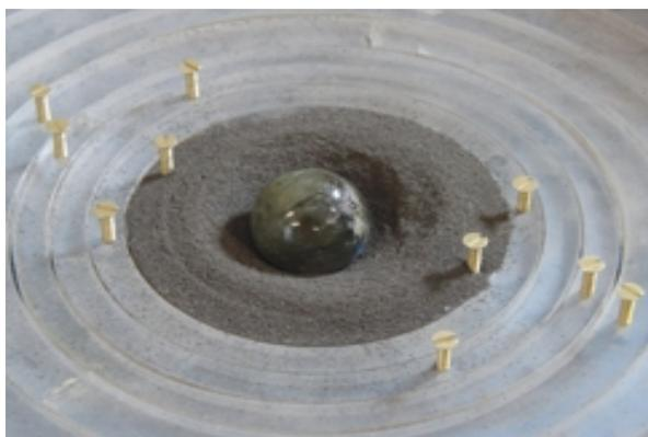
Figure 1: Impacts into JSC-1 target material create an ejecta blanket over the collection rings. High-speed, high-resolution imaging captures the spherical impactor colliding with the JSC-1 target material.
