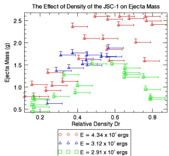
Figure 2: The effect of relative density of the target material JSC-1 on ejecta mass production is shown for three energy ranges. For each energy value, there is a range of maximum ejecta mass production.
