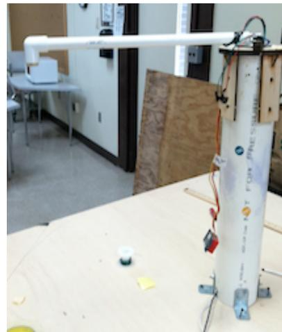
*Figure 1: Assembled robot with main body, arm, motor, temperature sensor, and ultrasonic range finder*
