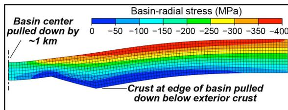
**Fig. 3** ABACUS finite element model showing exaggerated deformation (x20) of the crust following cooling of a subcrustal melt pool 100 km in radius. The basin center is drawn down ~1 km by the cooling melt, while isostatic equilibrium requires 4 km subsidence. A superisostatic anomaly is thus present. Deflection of thick crust at the basin edge produces a negative anomaly surrounding the basin.
