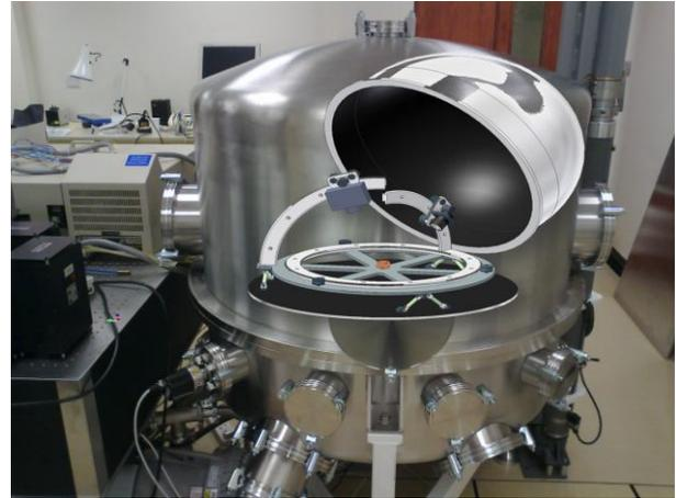
Figure 4: Goniometer CAD model superimposed on the vacuum chamber.
