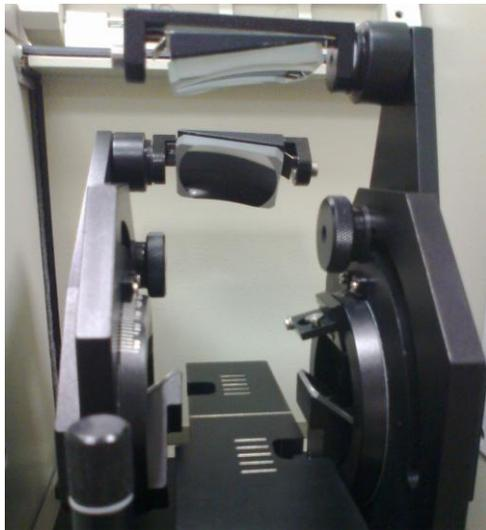
Figure 3: Multiple-angle reflectance accessory
