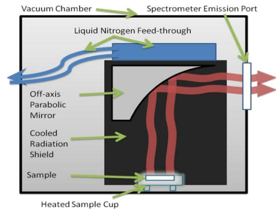
Figure 1: The heating-from-below setup
