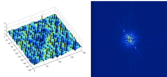
**Figure 2.** 2D Fourier transform magnitude diagram (right) of area shown in Figure 1-C, after detrending to remove overall topographic tilt (left). Bright points to upper left and lower right of center correspond to diagonal noise pattern. Brightness indicates higher amplitude. Distance from center indicates frequency of signal, where lower frequencies occur towards the center, and higher frequencies occur towards the edge.
