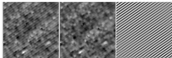
**Figure 3.** Cropped area as in Fig. 1-C displayed in grayscale (left); after performing the inverse FFT with a modified transform (middle); difference image (right) between the before and after correction images.
