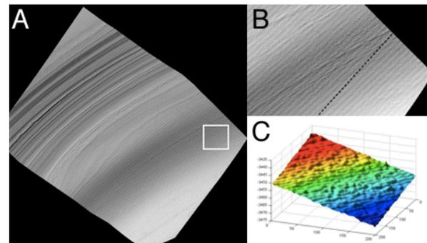
**Figure 1.** (A) Shaded relief image of HiRISE DTM DTEPC\_018870\_2625\_018910\_2625\_A01. (B) Detail of A showing subtle artifacts visible as periodic ripples that run parallel to black dashed line. (C) Subset of the DTM indicated by the white box in A, showing the noise patterns characteristic to this DTM. Elevation range in C (indicated by color blue=low, red=high) is ~30 m.
