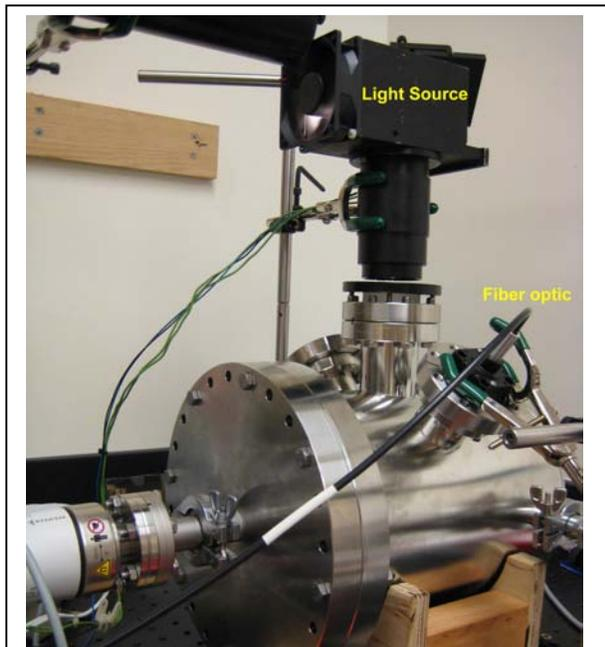
Fig 2. Environment chamber with light source (top) with an incidence angle of  $0^\circ$ , and fiber optic receiving the reflected light with an emission angle of  $30^\circ$ .
