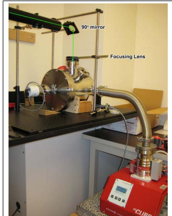
Fig 1. Space weathering experimental set up. Shown in green is the illustrated path of laser, which is redirected of 90° mirror and focused by a 300mm lens. Chamber is 8-inches tall by 10-inches long.
