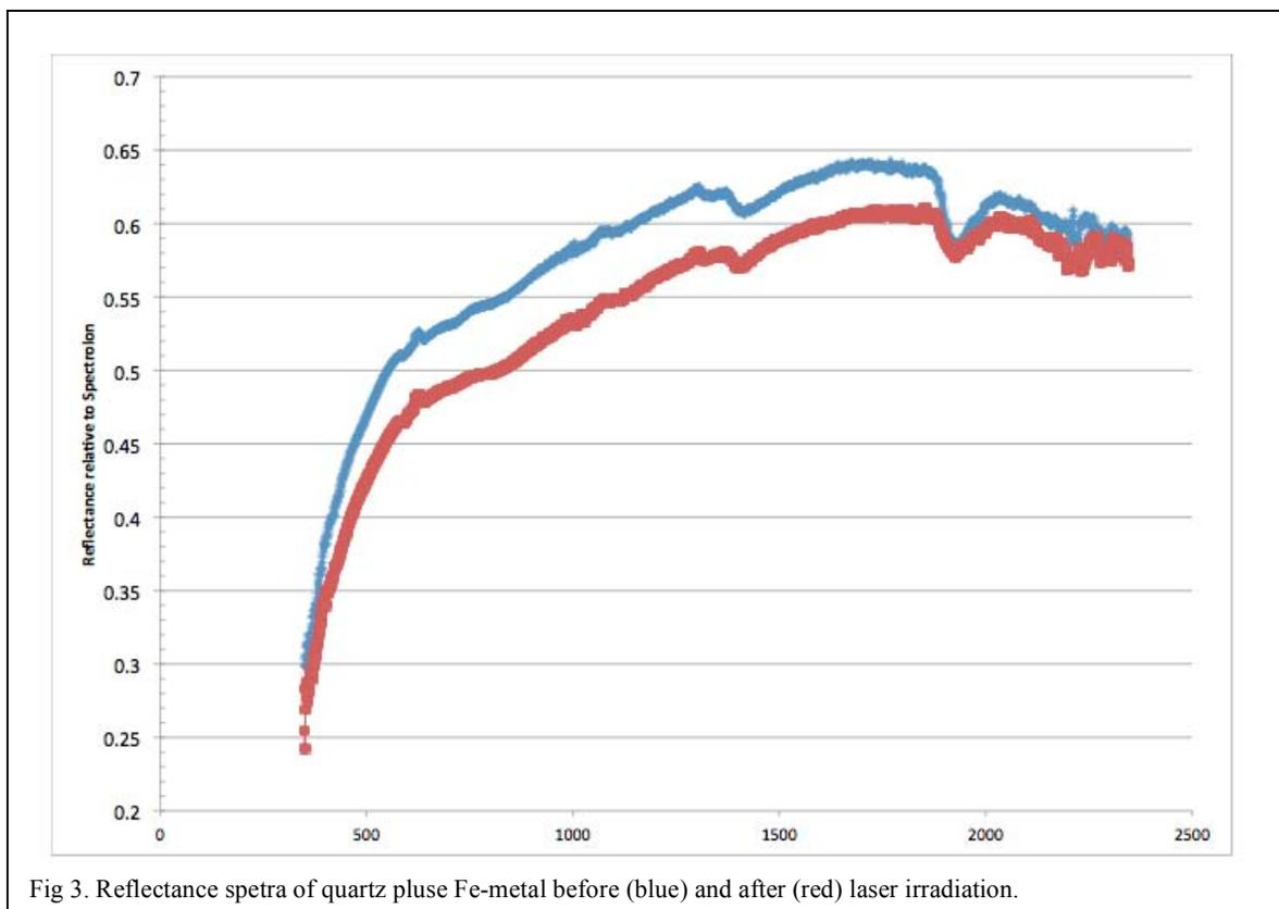
Fig 3. Reflectance spectra of quartz plus Fe-metal before (blue) and after (red) laser irradiation.
