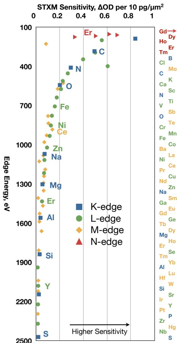
Figure 1: Theoretical edge jump for  $10 \text{ pg}/\mu\text{m}^2$  column density of all elements suitable for ALD with an absorption edge within range of ALS STXM beamlines 11.0.2 or 5.3.2.1. Important Stardust ISPE elements are labeled, plus Er which has 2 edges in the energy range.
