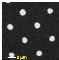
Figure 2: STXM Absorption image (740 eV) of 29nm- $\text{Fe}_2\text{O}_3$  and 95nm- $\text{Al}_2\text{O}_3$  ALD layers on holey  $\text{Si}_3\text{N}_4$  membrane, showing nm-scale homogeneity of Fe distribution.
