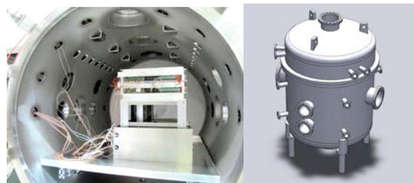
**Figure 2.** The Lunar Environment and Impact Laboratory chamber exterior (left) housing a dust-trajectory instrument for testing. This impact chamber will house UV, electron, and ion sources to simulate the variable plasma conditions on the lunar surface, and will act as a target chamber for the dust accelerator. The UHV chamber (right), designed for experiments of impact products, where ultra-high vacuum conditions are required.
