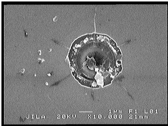
**Figure 3.** Scanning electron microscope image of an impact crater from hypervelocity impact onto fused quartz sample.
