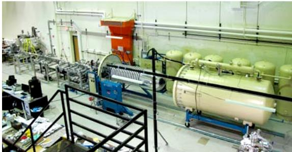
**Figure 1.** The 3 MV dust accelerator installed at in the CCLDAS Lunar Environment and Impact Laboratory. The accelerator is used to simulate the effects of dust impacts with speeds  $\gg 10$  km/s for micron sized projectiles. The facility will be also used to test and calibrate plasma and dust instruments, including the Lunar Dust EXperiment (LDEX) for the LADEE mission. The facility is now operational and available for the for impact studies.
