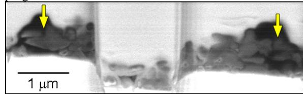
Figure 1. Backscatter electron image of the electron transparent cross-section containing presolar grains 3\_13a (left arrow) and 3\_13b (right arrow). The dark C cap is apparent under the Pt strap.
