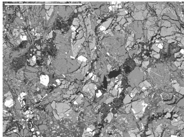
**Figure 4.** Petrography (top, in PPL) and BSE image of an altered Class 2 shocked basalt. Sample is same as the hand sample in Figure 3. “Feathery” textures in the BSE image are phyllosilicates. All needles are now maskelynite. Black voids running SW-NE are decompression cracks (Figure 3). Scale bar measures 1 mm.
