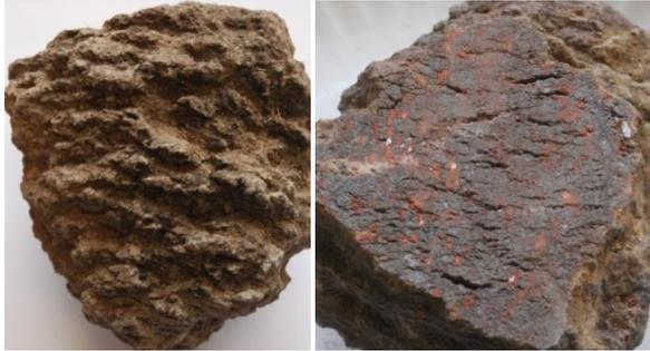
**Figure 3.** Natural and cut surfaces showing “decompression cracks” in a Class 2 shocked-altered basalt (~8 cm across) [3]. Petrography and SEM data shown in Figure 4.
