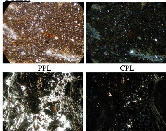
**Figure 2. Petrography of unshocked (top two) and shocked (bottom two) soils** in PPL (left) and CPL (right). The same view is on left and right with 5X magnification.
