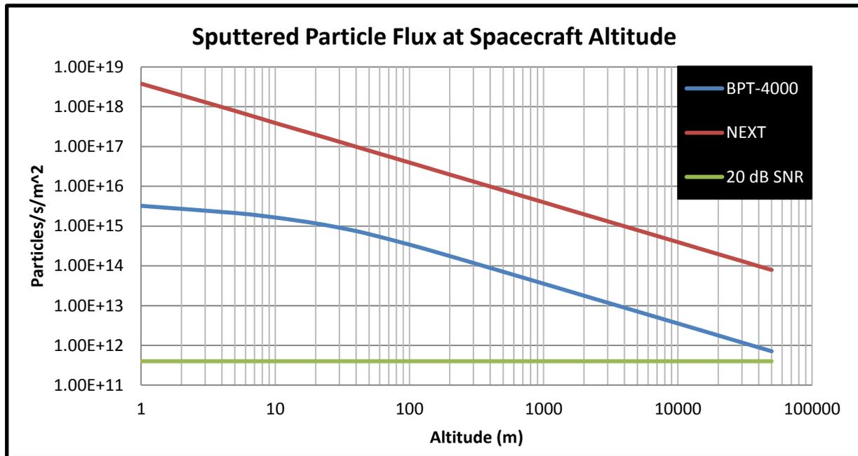
Figure 2 Expected EPI-SMS flux as function of altitude and electric propulsion type (BPT-4000, NEXT) operating with nadir pointing at full power on a MgO surface [7].
