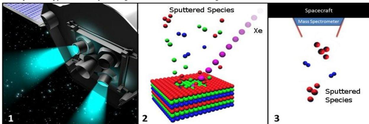
**Figure 1 EPI-SMS Operation.** 1. Spacecraft EP accelerates high energy Xe<sup>+</sup> toward body surface. 2. Xe<sup>+</sup> ions impinge on surface, sputtering species with 1-10 eV kinetic energy. 3. Sputter species arrive at spacecraft mass spectrometry for
