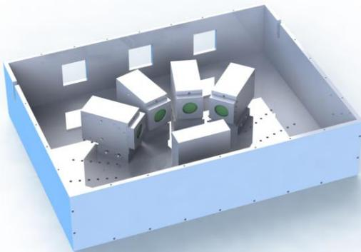
Figure 3: Schematic of light-flash experimental setup, with four photomultiplier tubes. Target is the slab at lower right; dust particles enter through the center square window.
