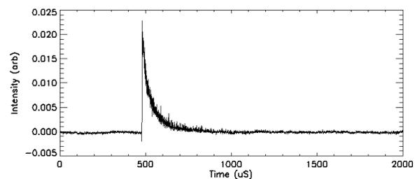
Figure 2: Light flash from an iron particle at 8.3 km/sec
