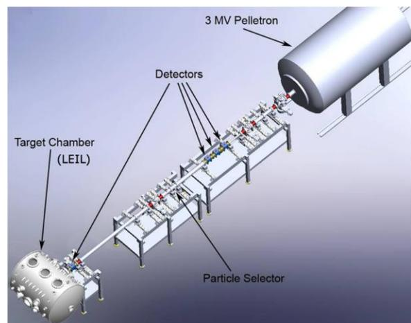
Figure 1: Dust accelerator at CCLDAS
