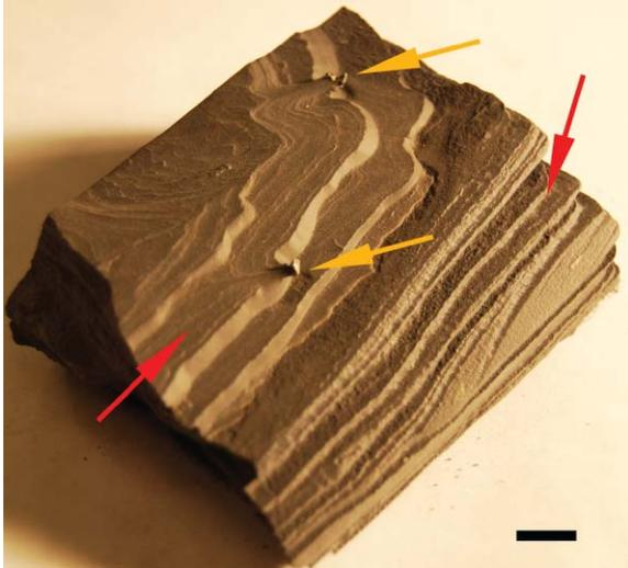
**Figure 2:** Erosional features observed after experiment with silt-rich black mudstones. Features include accentuated fine-lamina details/etching (red arrows), and pedestal formation (orange arrows). Scale bar 1 cm long.
