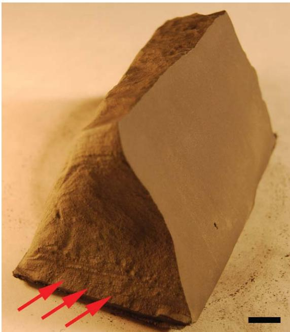
**Figure 3:** Erosional features observed after experiment with muddy siltstone. Red arrows point to accentuated fine-lamina that are etched out in fine detail. Scale bar 1 cm long.
