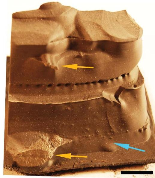
**Figure 1:** Erosional features observed after experiment with clay-rich black mudstones. Features include accentuated fine-lamina details/etching, pedestal formation (orange arrows), and polishing (blue arrows). Scale bar 1 cm long.
