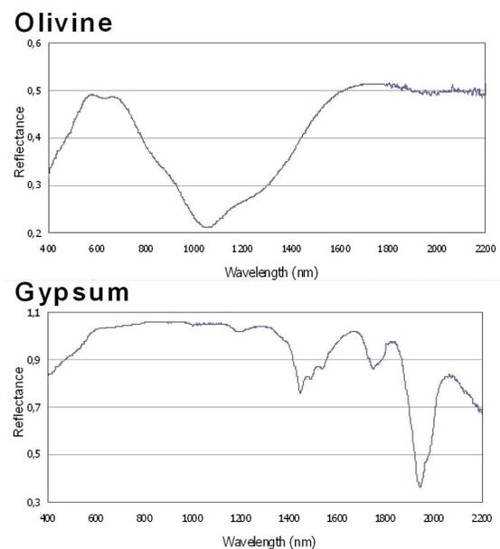
Figure 2: Example of prototype Ma-Miss instrument response signal taken in Olivine (volcanic rock) (top) and Gypsum (bottom). Credit: INAF-IAPS
