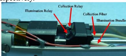
Figure 1: miniaturized optical head with the illumination and collection relays depicted.
