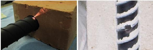
Figure 3: Two different moments of the Ma\_Miss Optical Head tests during the drilling. Left: The light beam comes out from the sapphire window on the Drill wall. Right: No evidence of dust on the window during the drilling Credit: *SELEX Galileo*
