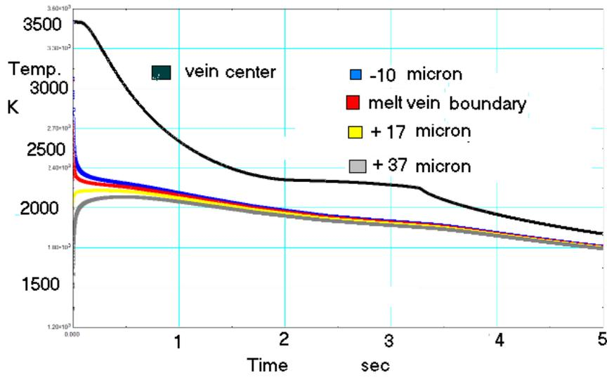
Fig. 1. Cooling calculation
