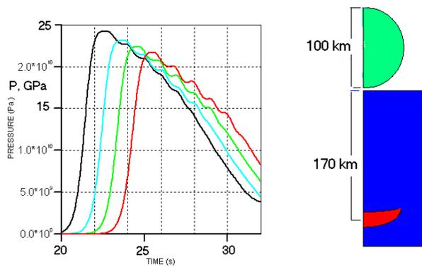
Fig. 3. Shock calculation for 7 Km/s impact
