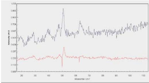
Figure 2. Raman spectra of the white and green materials identified as albite chlorite with minor bands from chlorite and oxides.
