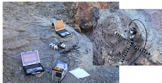
**Figure 1.** (Left) Raman instrument working at Los Azulejos area. (Right) detail of the Raman measurements at the blue-green minerals characteristics of Los Azulejos.
