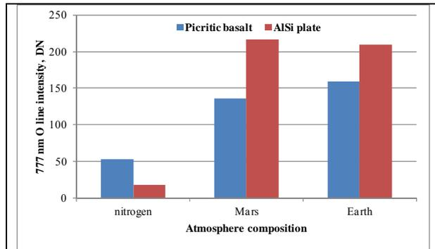
**Figure 2:** Intensity of the oxygen line around 8 mbar for 3 atmospheric and 2 target compositions.
