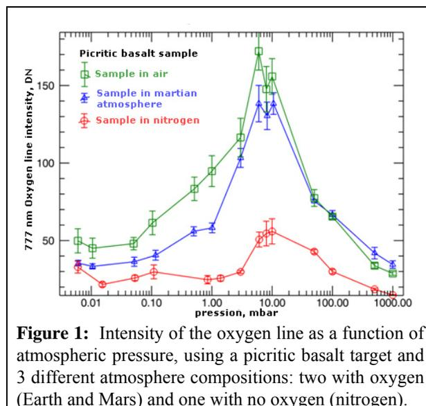
**Figure 1:** Intensity of the oxygen line as a function of atmospheric pressure, using a picritic basalt target and 3 different atmosphere compositions: two with oxygen (Earth and Mars) and one with no oxygen (nitrogen).
