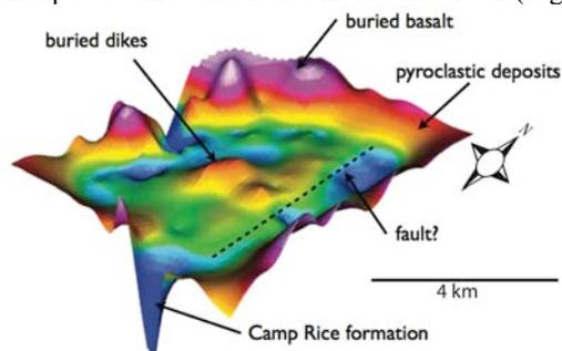
**Figure 2.** Magnetic anomaly map of Kilbourne Hole (3D oblique view).
