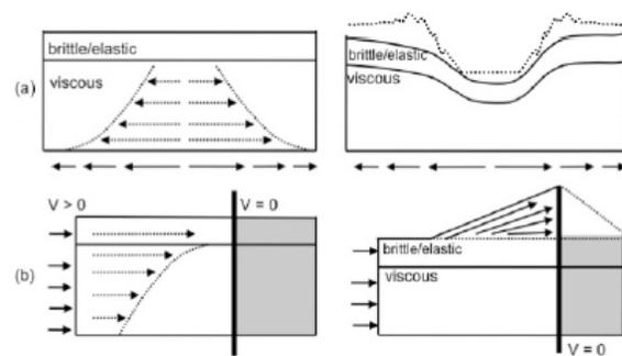
**Figure 2.** Two models. (a) vertical shear causes topography and uplift at sides; (b) flow into a zero-velocity “wall” causes build-up of material.
