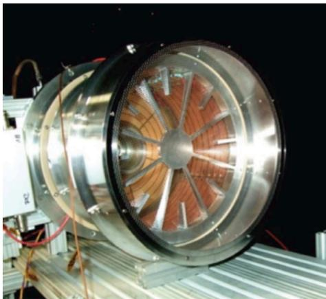
Fig. 3. The laboratory model of a modern, high resolution and low mass dust spectrometer instrument.
