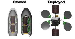
Advanced Modular Power System (AWF-G). The 702 SP for deep space is designed to be able to use the Advanced Modular Power System (AMPS) solar array, producing high (multi Kw) power levels with significantly lower system mass (specific power densities of ~130 watts/kg) than current solar power system technologies. This power can be used to operate the SEP system
