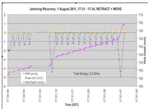
**Figure 2. Automated detection and recovery of a down-hole jam by Icebreaker.**
