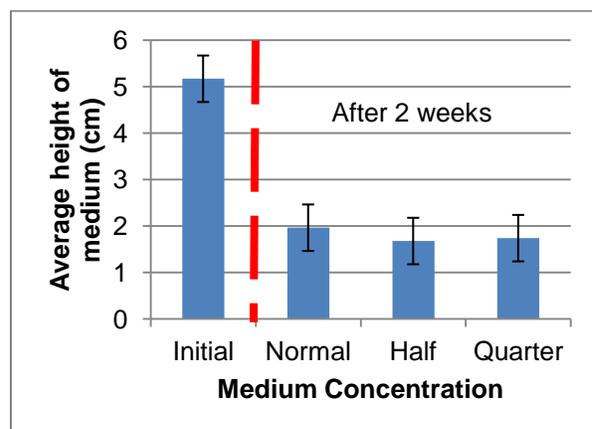
**Figure 2.** Height of methanogen growth medium at different concentrations, following two weeks at room temperature and 130 mbar.
