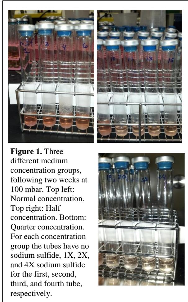
**Figure 1.** Three different medium concentration groups, following two weeks at 100 mbar. Top left: Normal concentration. Top right: Half concentration. Bottom: Quarter concentration. For each concentration group the tubes have no sodium sulfide, 1X, 2X, and 4X sodium sulfide for the first, second, third, and fourth tube, respectively.
