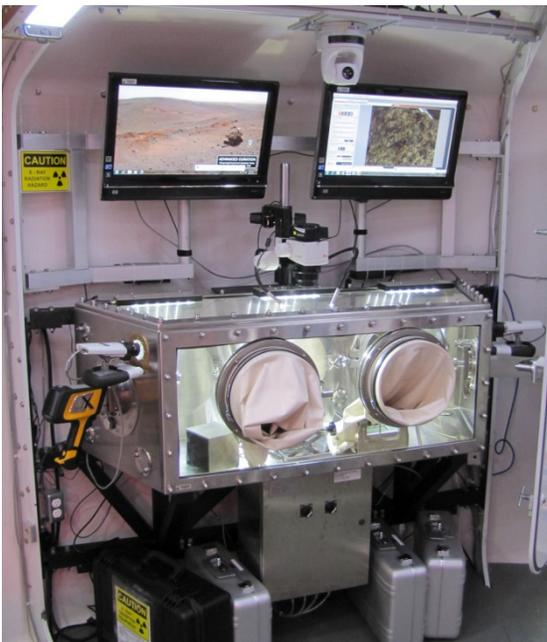
Figure 1: GeoLab glovebox integrated into NASA's Deep Space Habitat Demonstration Unit.
