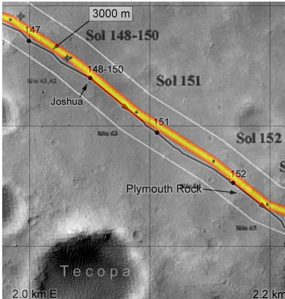
Figure 3. Comparison of Spirit route maps - this study (black line, large dots) and the JPL MER website route map (yellow line, small dots). Position errors are 5 to 10 m across the track, about 25 m along the track, the JPL map lagging the true position..
